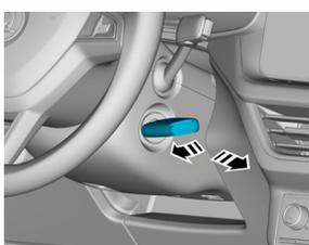
1. Turn the ignition key to the "OFF" position and take out the key
