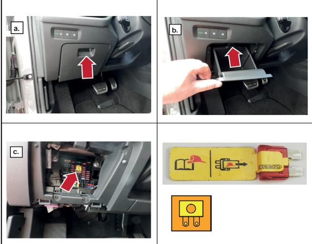
**Optionally deactivate the high-voltage system in the vehicle interior.**
