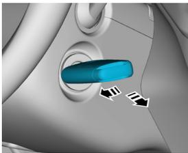
Turn the ignition key to the "OFF position" and remove it
