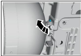
Close valve on gas tank No. 2 in direction of arrow using handwheel -T50026-(ŠKODA special tool) or pliers.
