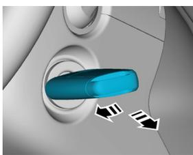
1. Turn the ignition key to the "OFF" position and take out the key
