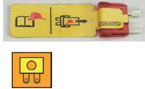
**Optionally deactivate the high-voltage system in the vehicle interior.**
